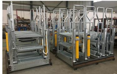
Folding stairs is specially designed to provide safe and efficient means of access between a loading platform and road or rail tankers.
